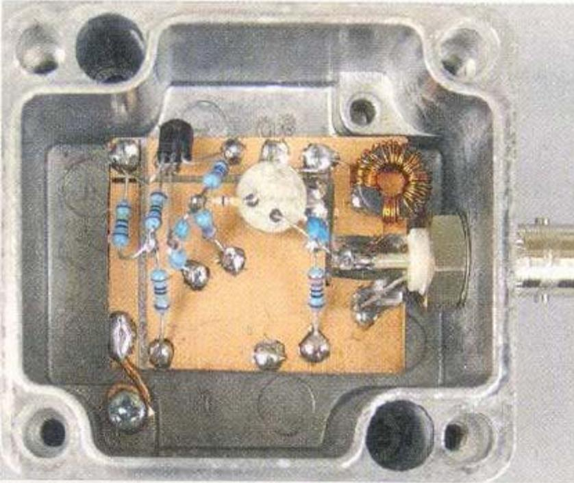
*Photo 5 - Diecast-box Mini-Whip.*
