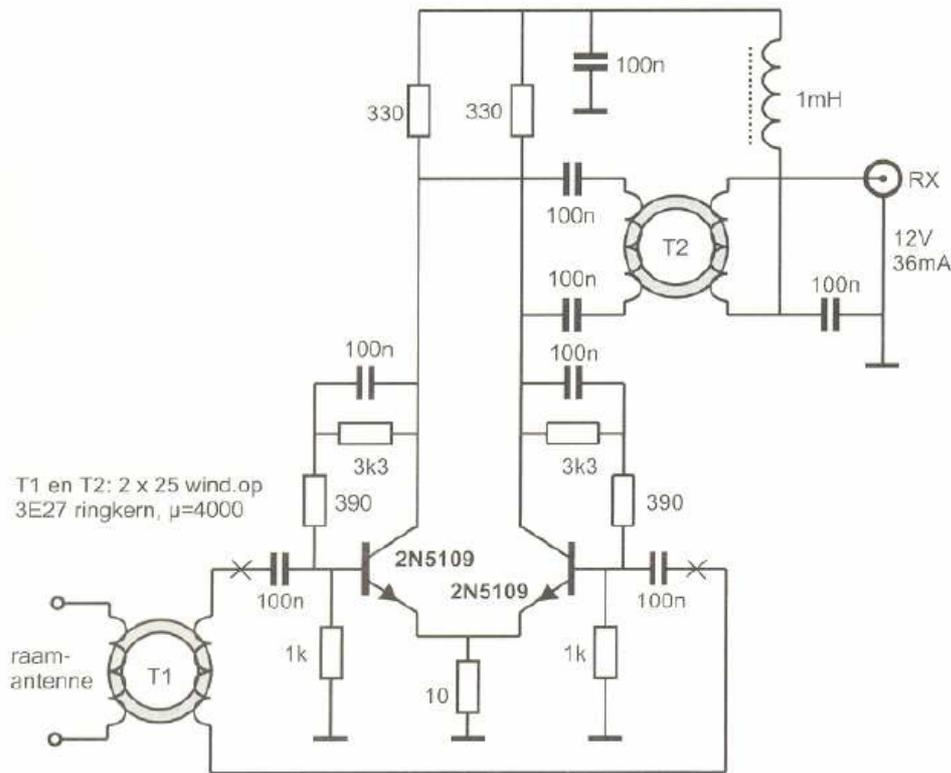
Figure 1 - Balanced active loop antenna.
