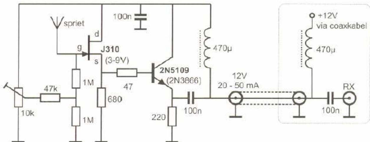
Figure 3 - Experimental version of the Mini-Whip.
