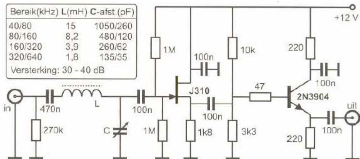
Figure 5 - Tunable preamplifier.
