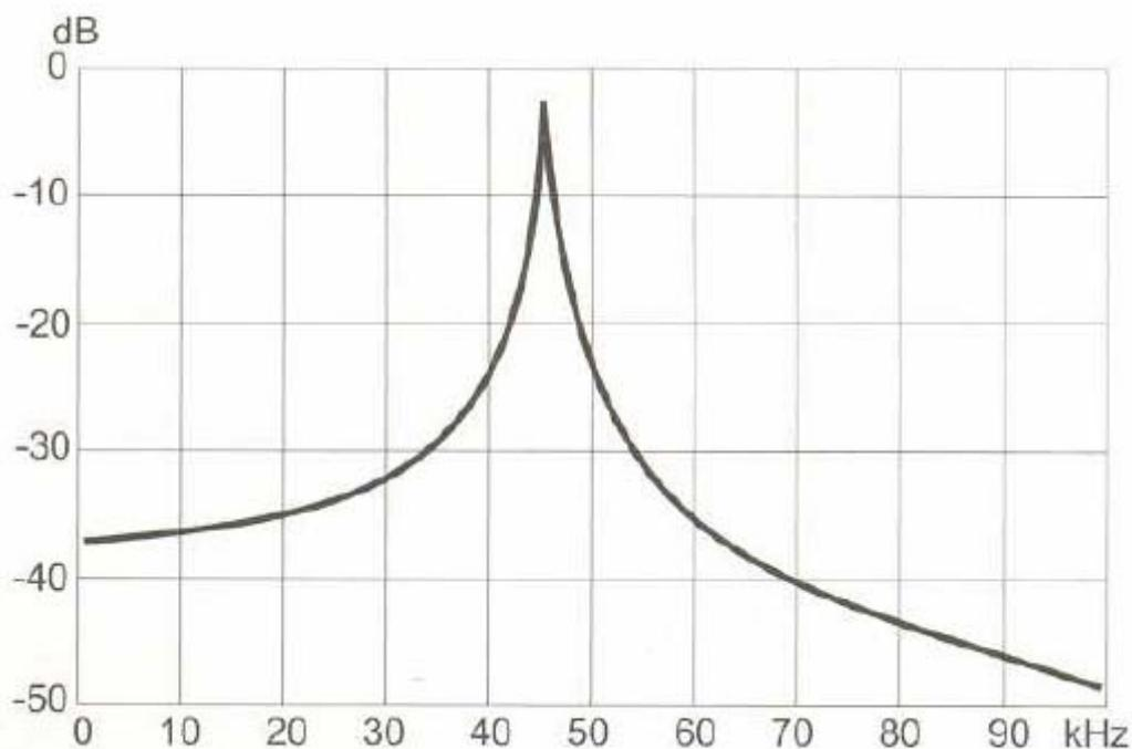
Figure 6 - Frequency response for the circuit in Figure 5.
